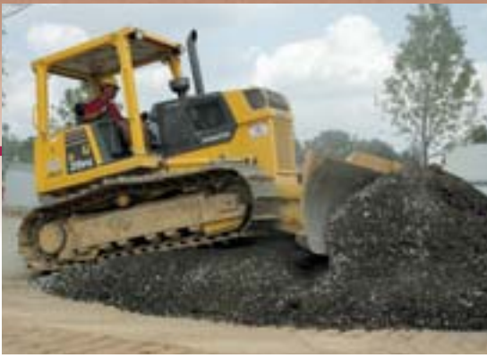
Foreman Tom Jost uses the company's new Komatsu D39PX-21A Komstat II dozer to move fill dirt at a new car dealership jobsite in Upper Saddle River, N.J.
